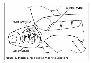
Caution should be taken when handling the connections to the magnetos. Magnetos can generate several hundred volts on their P-Leads that can provide sever shock hazard to the installer.
