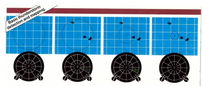
**B-1** To test, turn power/mode switch to "ON", set range at 100 or 200 nm. (No test pattern appears at 25 or 50 nm ranges.) Allow 30 seconds for warm-up, then push "TST" button. If functioning properly, a small cluster of dots appears at 1:30 and 100 nm (inner circle at 200 nm setting, outer circle at 100 nm setting). Holding "TST" button in generates several dots per second. Press "CLR" button after completing test.
