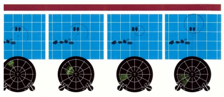
sircraft turns to the right to if the thunderstorms. When a completed, push "CLR" he screen will map the new of thunderstorm activity the aircraft heading. When er ranges can be used, more ecisions can be made to around thunderstorms.
