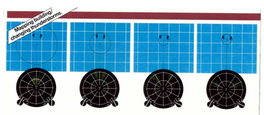
D-1 With range set at 200 nm, two moderate thunderstorms appear, at 11:30 and 12:30. Each is approximately 25 to 30 nm wide. Each is centered about 90 nm from aircraft. Radial spread from each indicates both are of moderate intensity.
