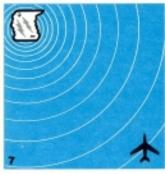
7 The radiated electromagnetic signals from electrical discharges are powerful enough to be received and detected at great distances. Your model WX-10A can receive signals from discharges more than 200 nm sway.
