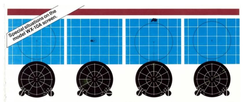
A-1 Randomly scattered dots. Possible causes: Turning electrical switches on or off, atmospheric instability associated with cumulus clouds, developing or dissipating thunderstorms, etc. If screen shows this situation, push "CLR" button. Watch screen for developing clusters of dots which indicate thunderstorm activity.
