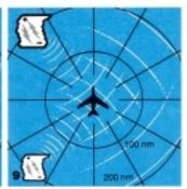
9 To effectively map the location of the thunderstorms, the radiated signals being received must be analyzed for both azimuth (direction) and range.
