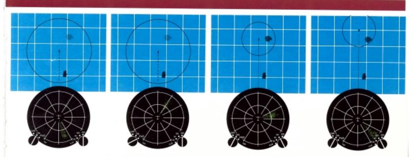
C-1 Display shows weak thunderstorm at 1:00, about 100 nm from aircraft, and severe thunderstorm at 5:30, about 150 nm away. Fewer dots and less radial spread at the location of the 1:00 thunderstorm indicate a lesser rate of occurrence, hence, a weaker thunderstorm.
