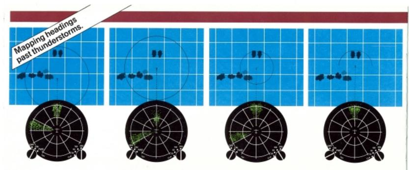
F-1 With range set at 200 nm, two severe thunderstorms appear almost as one cluster of dots off the nose of the aircraft, centered about 180 nm away. A second cluster at 9:30 indicates a system which contains several severe thunderstorms. Thunderstorm conditions change rapidly. Avoid premature judgment when thunderstorms are mapped near the outer circle on the 200 nm range.
