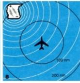
8 Since the signals radiate out in all directions and your model WX-10A can receive the signals from all directions, thunderstorm activity can be mapped 360° around the aircraft.
