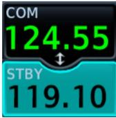
The selected STBY window turns cyan when the knob is used to change the STBY frequency.
