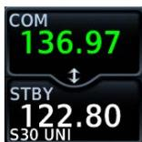
Standby COM frequency tunes to either the airport CTAF or tower frequency (if the active frequency is not already tuned).
