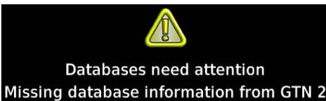
A message informs you when database information from the indicated LRU is missing. This appears when an LRU is not powered on during start-up.
