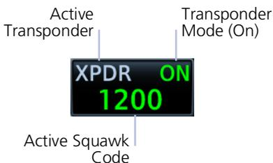
Tapping the **XPDR** key activates the IDENT function for 18 seconds. This signal distinguishes the transponder from others on the air traffic controller's screen.
