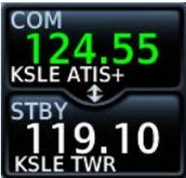
Enabling this option displays the facility identifier and frequency type for active and standby frequencies.
