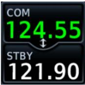
VHF COM transceiver controls are accessible via the selectable standby (STBY) frequency window.
