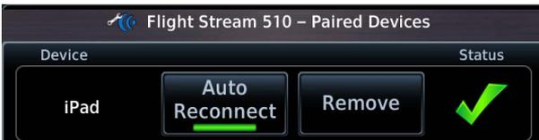
To enable automatic connection between the unit and a paired device at power up, tap **Auto Reconnect**.
