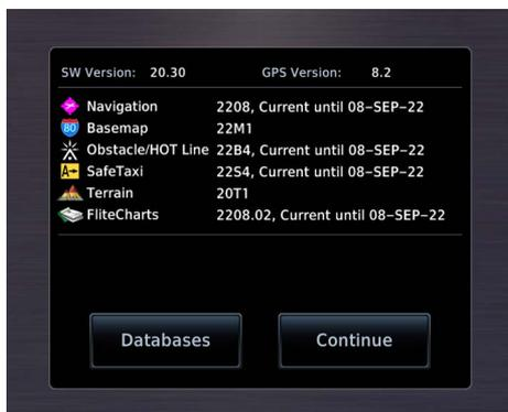
Start-up pages present the unit software versions and the name and status of all installed databases.
