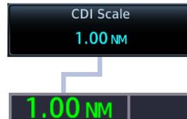
**CDI scale is set to “Auto” (default).** At the default setting, the scale sets to 2.0 NM during the en route phase of flight.
