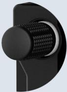
Turning the volume knob while the NAV frequency window is activated adjusts the radio’s volume percentage.
