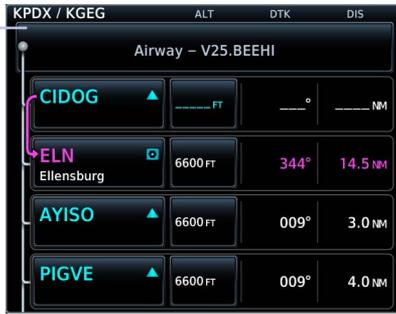
All airways begin with an indicator field and end with an exit identifier.
