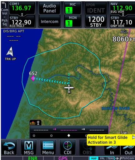
The "Hold for Smart Glide Activation" control label appears near the bottom of the display when you activate the feature using the **Direct To** key.
