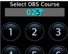
When active, this function allows you to set the desired course To/From a waypoint using the provided controls or with an external OBS selector on HSI or CDI.
