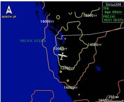
Color-coded contour lines indicate the altitude of the freezing level.
