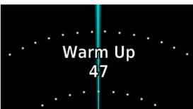
A warm-up period initiates upon power up (GWX 68 only). Duration varies depending on how long the radar is off. The radar begins transmitting once warm-up is complete.
