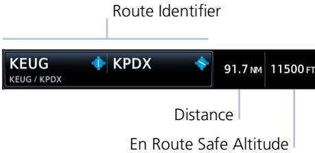
In addition to the route identifier, these units display the route distance and en route safe altitude.
