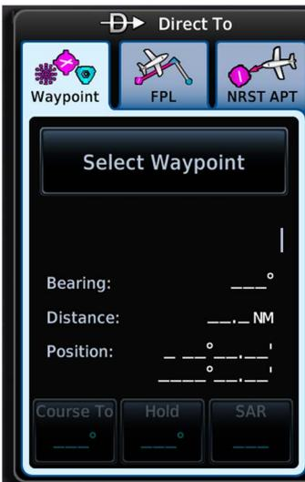
Pushing this bezel key opens a slide-out window. Search tabs provide three different methods of waypoint selection.
