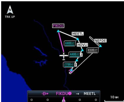
The active altitude constraint is the altitude to which VNAV is currently providing guidance.
