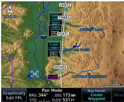
Displays altitude and/or speed<sup>1</sup> constraint labels within the flight plan.
