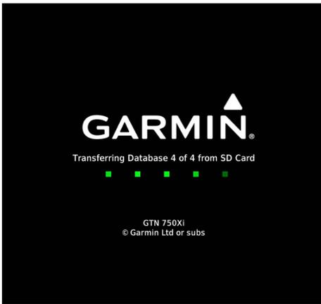
The unit detects when an SD card with recommended databases is present in the slot. Updates occur automatically at power up.
