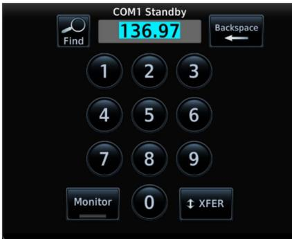
Tapping **STBY** opens the control panel for the indicated radio.
