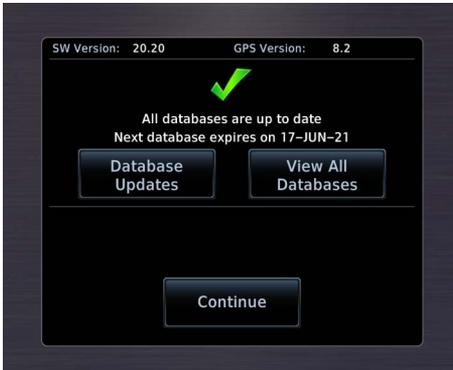
A message on the primary GTN Xi informs you when the databases on all capable avionics are up to date.
