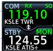
Monitor mode is useful when you want to listen to a recorded broadcast (e.g., ATIS) on the standby channel, but still receive control tower transmissions on the active channel.
