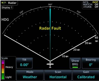
Caution messages alert you when there is a weather radar failure. For a list of possible radar alerts, refer to the annunciations table in this segment.
