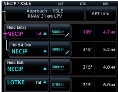
If VNAV is enabled, each hold leg is accompanied by a separate altitude constraint value.
