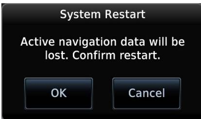
*Confirmation is required as active navigation data will be lost during system restart.*
