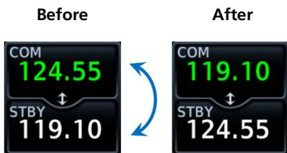
The transfer (or *flip-flop*) function allows you to swap the active and standby frequency values.
