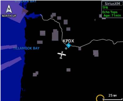
Depicts the location, elevation, and direction of NEXRAD radar echoes. This information is useful for gauging storm intensity in a relative sense. A higher radar echo means a stronger storm updraft.
