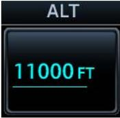
Altitude constraints are either entered manually into the active flight plan, or automatically retrieved from the published altitudes in the navigation database. GTN automatically uses altitudes loaded with arrival and approach procedures (up to and including the FAF) for computing vertical deviation guidance.
