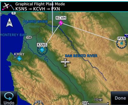
The temporary flight plan adjusts to show the new route.
