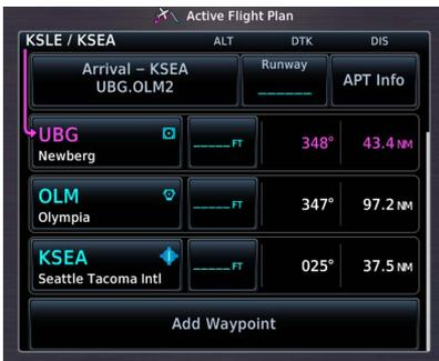
Deferring runway selection displays a series of dashes on the corresponding leg of the active flight plan. Selecting **Runway** re-opens the runway list.
