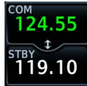
COM radio operates in the aviation voice band, between 118.000 and 136.975 MHz, in 25.0 kHz steps.
