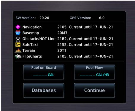
GTN Xi stores preset fuel amounts for estimated full and tab amounts. These settings may not be editable if the unit is interfaced with a digital fuel computer.
