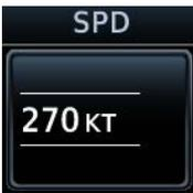
Like altitude constraints, speed constraints are either entered manually into the active flight plan, or automatically retrieved from the published airspeeds in the navigation database. GTN automatically uses airspeeds loaded with arrival, approach, and departure procedures (up to and including the FAF).
