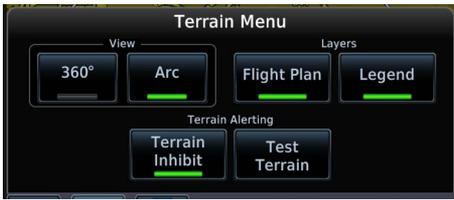
The **Terrain Inhibit** control is accessible via the terrain pop-up alert or the Terrain page menu.
