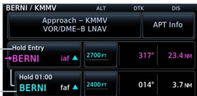
Not all published holds support a Hold Exit leg. Some show only Hold Entry and Hold legs. In this case, the Hold leg will remain active until crossing the hold fix for the final time.
