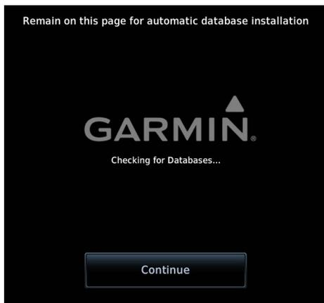
*"Checking for Databases..." annunciates as the unit checks for available database updates.*
