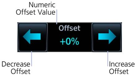
If the unit is wired for audio output, set the sidetone volume offset to the preferred level. By default, the offset value is set to zero percent.
