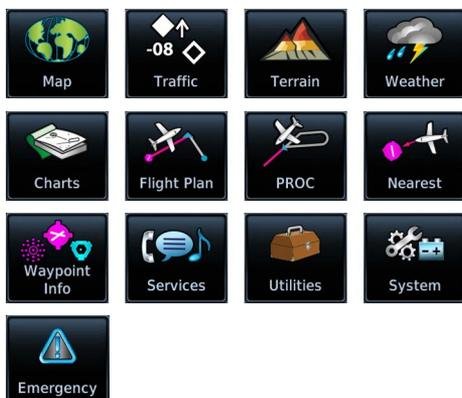
Tapping one of these icons opens the corresponding application. Some apps provide additional icons for accessing functions on subpages (e.g., System, Utilities).
