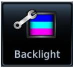
Depending on configuration, display brightness is controlled using inputs from the built in photocell, aircraft dimmer bus, or both.
