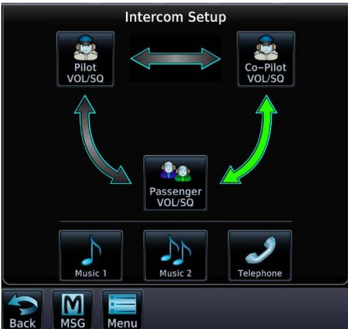
Tap the arrow between the intercom recipients. When the arrow is green, it indicates communication is active between the recipients.
