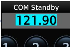
Enter a new standby frequency using the provided data entry keys or by turning and pushing the control knob.
