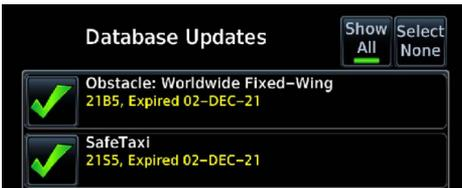
Previous database versions appear as non-recommended databases in the standby list. They remain available for manual install until a newer version transfers to the internal Standby storage.
