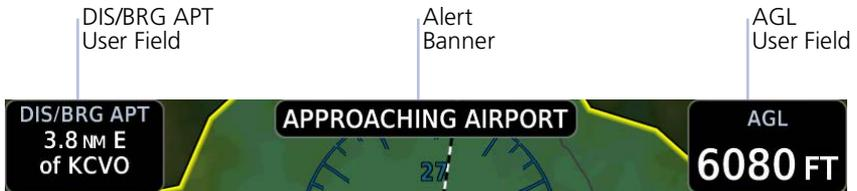
If previously configured by the pilot, these two user fields remain in the same location once Smart Glide is activated. If not configured, they will appear in the upper corners as shown. If only one field is configured, the other will appear in the upper left or right corner.
