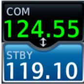
You may enter a standby frequency using the data entry keys on the COM Standby control panel or by turning the control knob.
