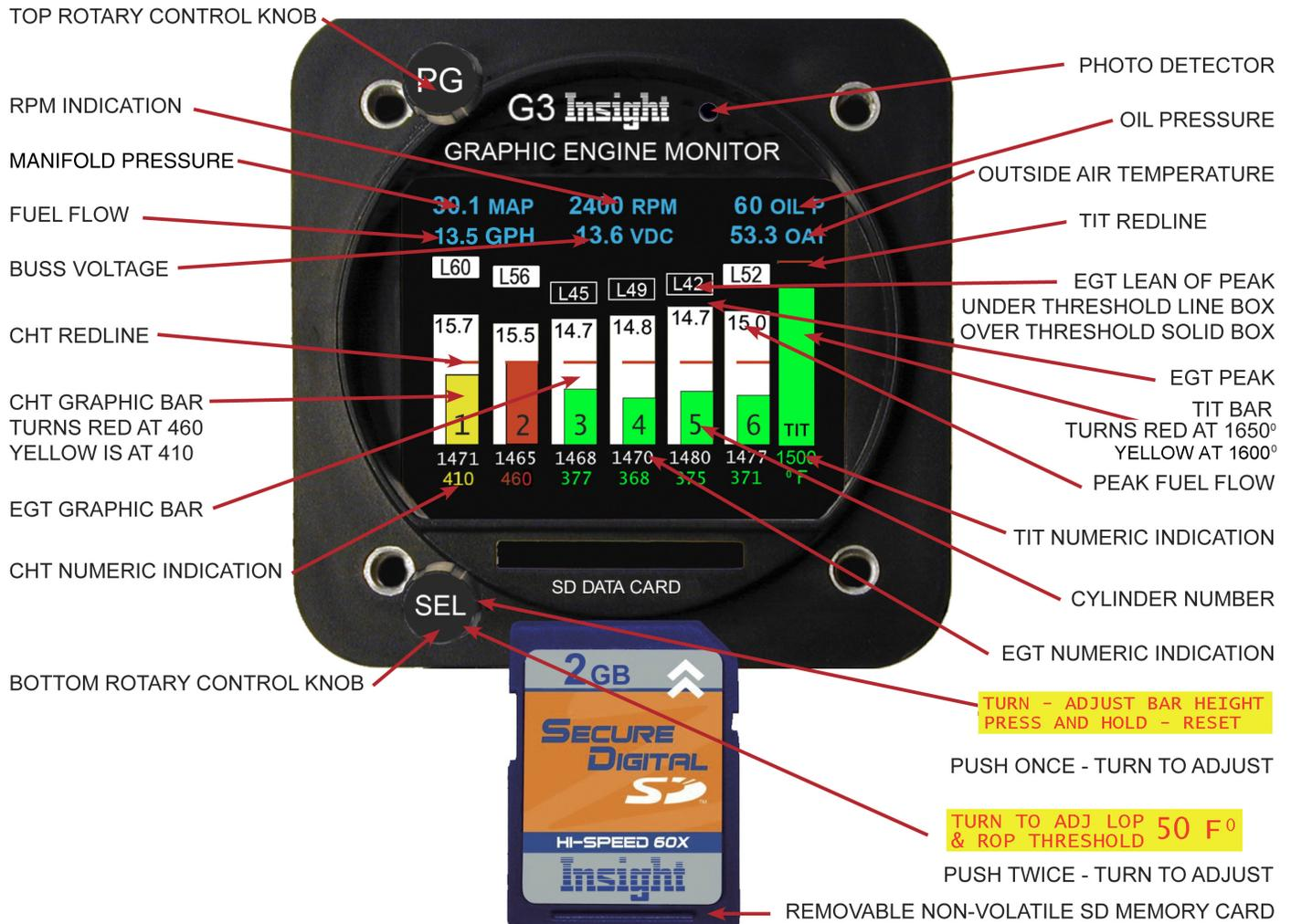
The instrument has two control knobs that operate combination rotary and push button switches. The top knob in general controls screen selection while the bottom knob controls items within the given screen.
